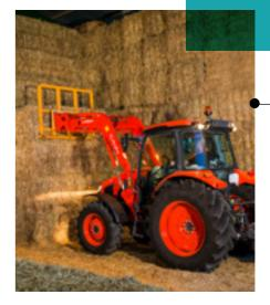
Whether you need to work with a manure fork, pallet fork, bale fork, or a bucket – each of them can be quickly attached and removed from the LA1854 front loader thanks to the standard EURO hitch interface.
